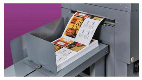
Differentiation for high-quality prints is a premium, and no longer available only to the production market! The Duplo DDC-810 is an offline UV spot coater targeted toward midto entry-production arenas. Compact and user friendly, it achieves precise, valued UV coating by an accurate CCD reading system and inkjet control. Add value to your print with a layer of spot UV embellishment that you can touch and feel.
