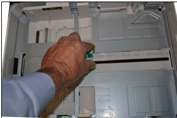
Above and below: In order to adjust the 520-sheet paper drawers to accommodate different paper sizes, the user squeezes and slides these green guides into place. BERTL found it easy to adjust all the paper drawers.
